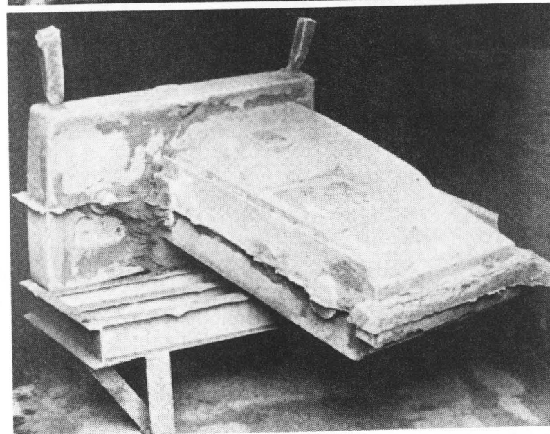
Top: Match-plate removed, cores set in place. Bottom: Completed casting
