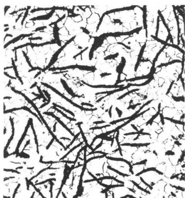
Flake Graphite and Spherical Graphite 250x
